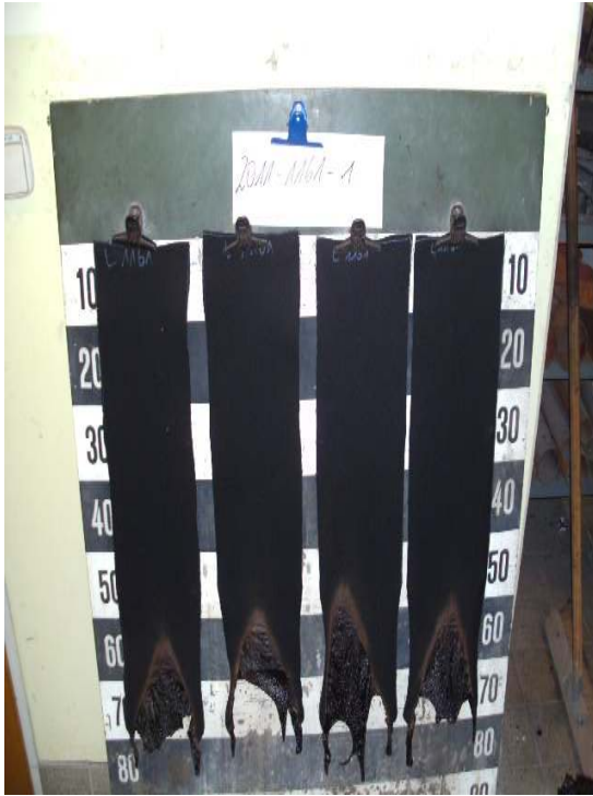
Appearance of sample A after the "Brandschacht" test
